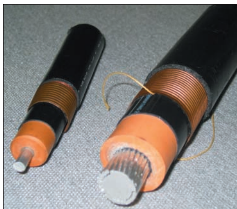
Examples of underground electric cable used by Choptank. The wire is surrounded by ethylene propylene rubber (EPR).
